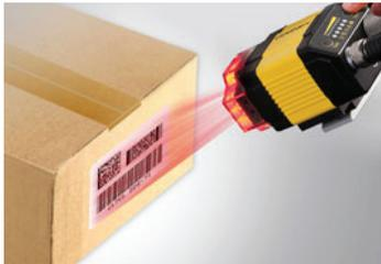
DataMan readers feature various trigger modes during image acquisition. For example, a reader in burst mode can decode and output multiple codes from a sequence of images or in continuous mode can be set to take as many images as necessary to locate a specified number of codes.
